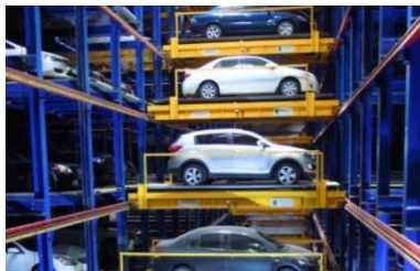
Slide Elevator Mechanical Parking System (PPY)
