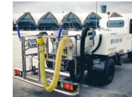
Toilet Service Units
